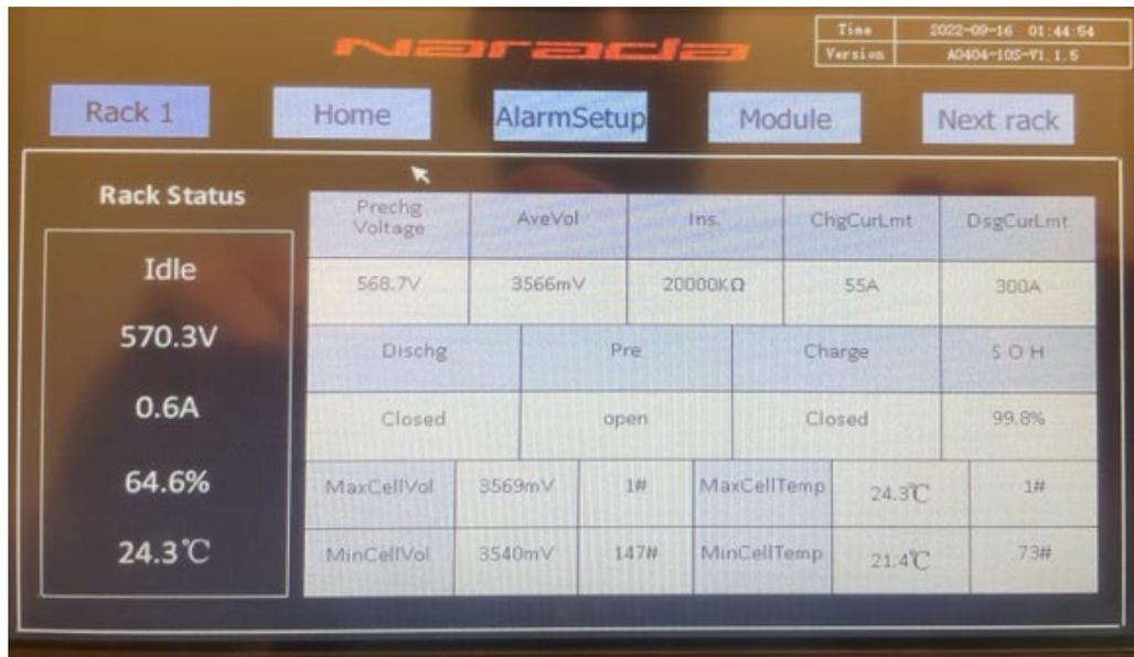
Touch the **Module** button to enter the BMU information collection interface, which contains the cell voltage and temperature information collected by the BMU. RACK1 M1 shows the
