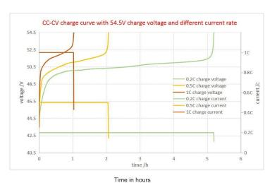
Fig.2-2 Charge curve at different current limitation of FEN4850 battery
