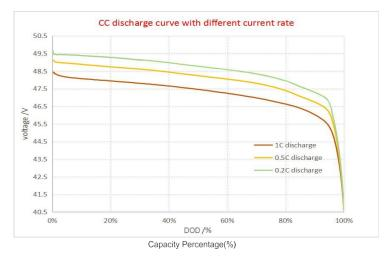
Fig.2-1 Discharge curve at different constant current of FEN4850 battery
