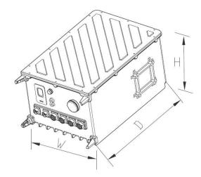
Fig.1-1 Structural Drawing of FEN4850 Batteries
