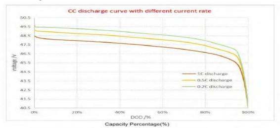
Fig.2-1 Discharge curve at different constant currents of NPFC / MPLhE series
