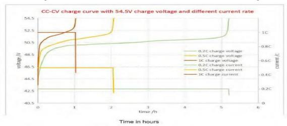
Fig.2-2 Charge curve at the different current limitations of NPFC / MPLhE series
