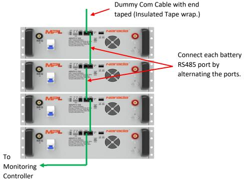
The last battery in each rack has an empty RS485 port, it needs to be connected with a cable with RJ45
