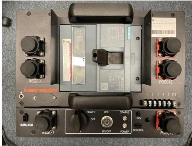
**Control Box with internally installed BCU**
