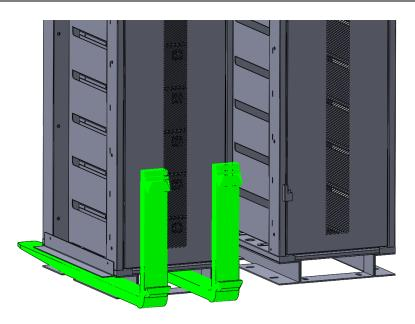
Slightly lift the rack and reposition it adjacent to the one already in place. Remove the angle bracket on the left side of the second rack and anchor it to the floor. Anchor  $2^{nd}$  rack to the floor
