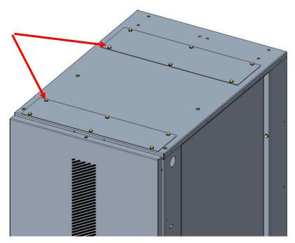
Remove the front cover from the CLB and Place the box on top of the cabinet and ensure the mounting holes are aligned.
