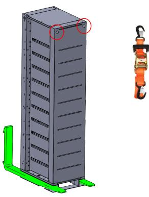
Position the first rack in place. Remove the angle brackets from both sides.
