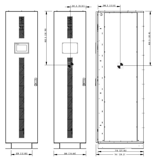
Fig 4-1 Front and Side Views of the Standard 10-Module Rack
