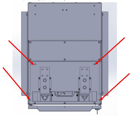
Connect the busbars to the control box output terminals using provided hardware. Tighten the Bolts and Nuts to 25Nm torque.
