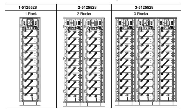
6.1.1 For a standard 10-module rack, the bottom module (#10) shall be place first.
