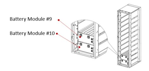
Fig 6-2 Battery Module Arrangement from the Bottom
