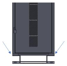
Secure the rack with the anchoring bolts to the floor.
