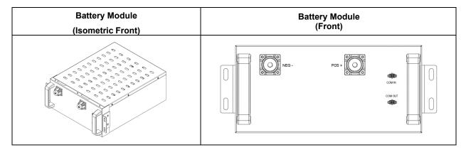
Fig 3-3 Front and Isometric Views of the Battery Modules
